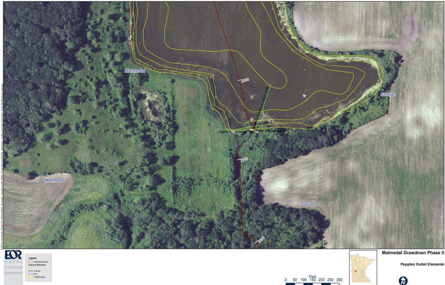
Figure 12. Pepples Slough Outlet Alignment
